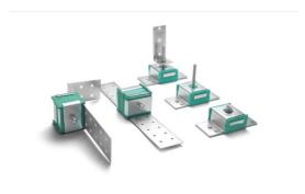
Range designed for the floating suspension of soundproofed walls. Sylomer® avoids the transmission of vibrations while providing optimal acoustic results. They have a "FAIL SAFE" rugged metal structure, which is overload-proof. Recommended for applications where fire or impact resistance is necessary. These mounts are also suitable for the isolation of vertical pipes, or any type of lightweight ducts that need to be isolated.
